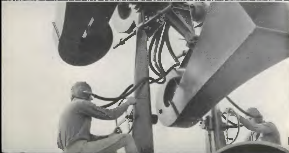
Giant sound locators on the alert for the Naval fleet planes during joint maneuvers near the Panama Canal.
