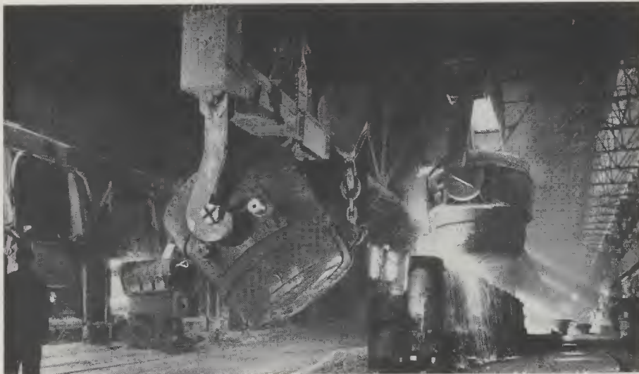
Molten iron and steel being poured from ladles forming controlled quality steel ingots.
