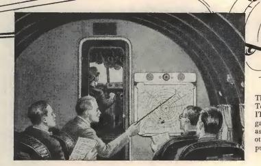
The interior of the "Flying Laboratory" of Federal Telecommunication Laboratories, a division of IT & T, is a veritable airborne workshop. Here, navigation aids for use at short and very long distances as well as for low approach and landing, and many other experimental radio and electronic devices are put through their paces under "in-service" conditions.
